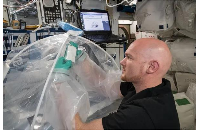
Astronaut Alexander Gerst experimenting with cement made with the mock lunar soil.
